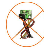
No charge controller unless 20 Watt panel or above
